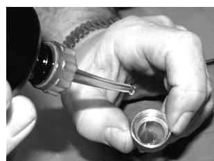
**⚠ Use oil as couplant: Hydrated couplants (e.g. ECHOTRACE) are not well-suited for application on the inner side of the membrane since they tend to dry out and may cause air bubbles between probe and foil.**
